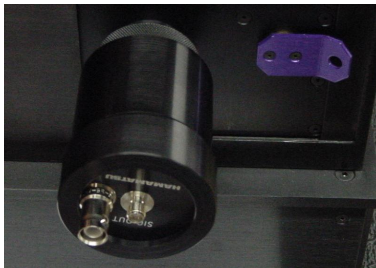
Figure 6.11 ChronosBH equipped with the MCP model R3809U mounted on the left emission channel.
