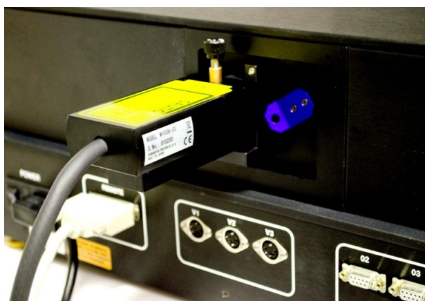
Figure 9.5 Connection of the laser to the Chronos.
