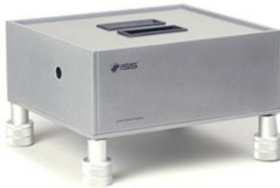
Figure 9.14 Unit A452 for conditioning the reference signal from multiphoton lasers.
