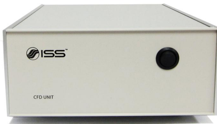
Figure 9.15 Unit A452 for conditioning the reference signal from multiphoton lasers.
