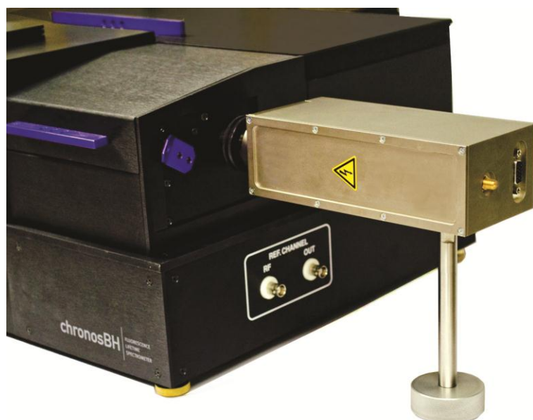
Figure 6.10 ChronosBH equipped with the hybrid PMT model R10467U mounted on the right emission channel.
