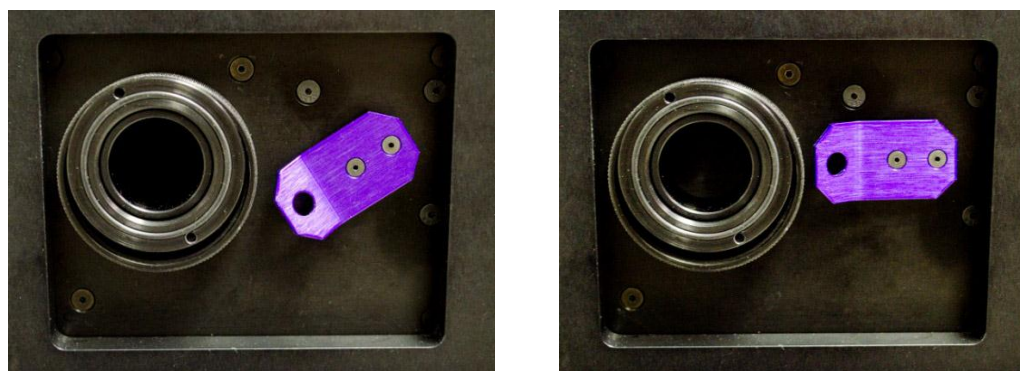
Figure 2.8 Excitation shutter OPEN (left) and CLOSED (right)
