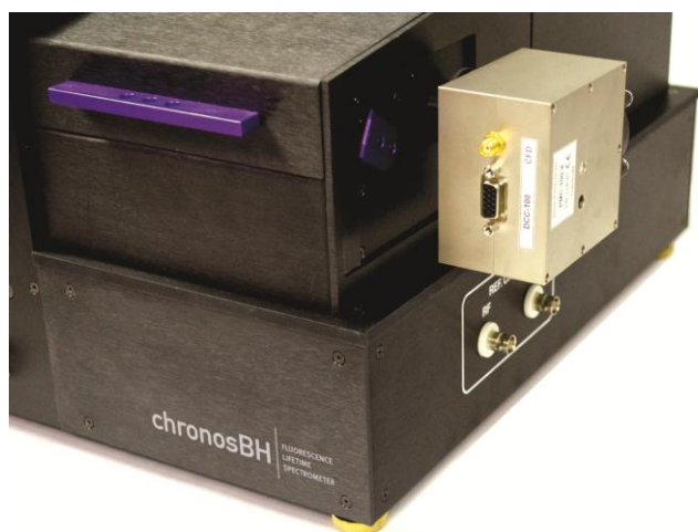
Figure 6.8 ChronosBH equipped with the PMT model PMC-100-4 mounted on the right emission channel.
